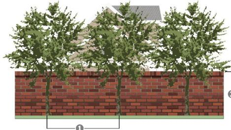
1: CANOPY TREES 20-FOOT ON CENTER; 2: MINIMUM SIX (6) FOOT MASONRY WALL;
