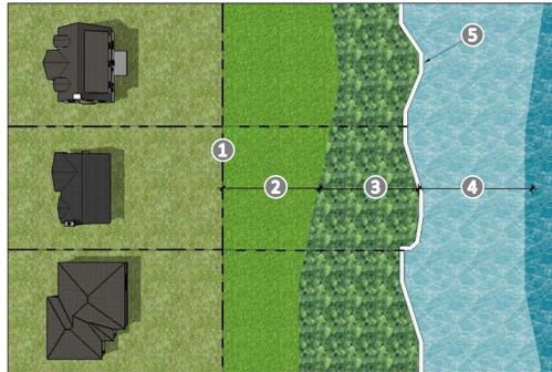
1: REAR PROPERTY LINE/TAKE LINE; 2: 438.0 ELEVATION ZONE; 3: 435.5 ELEVATION ZONE; 4: 425.5 ELEVATION ZONE; 5: SEAWALL;
