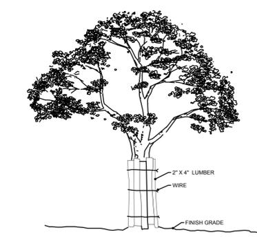
WHERE A PROTECTED TREE REMAINS IN THE IMMEDIATE AREA OF INTENDED CONSTRUCTION AND THE TREE MAY BE IN DANGER OF BEING DAMAGED BY CONSTRUCTION EQUIPMENT OR OTHER ACTIVITY, THE CONTRACTOR OR SUBCONTRACTOR SHALL PROTECT THE TREE WITH 2\"/>
