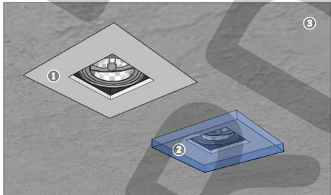
1: FLUSH LENS (I.E. FULLY RECESSED); 2: PROJECTING LENS (I.E. NOT FULLY RECESSED); 3: CEILING
