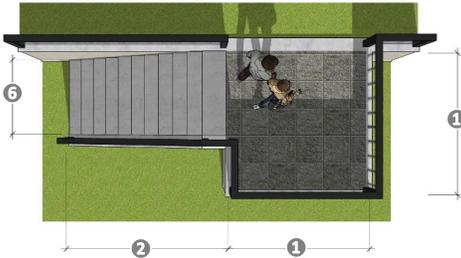
1: MINIMUM OF EIGHT (8) FOOT BY EIGHT (8) FOOT LANDING; 2: VARIABLE LENGTH STAIRCASE; 3: WROUGHT IRON OR BLACK TUBULAR STEEL; 4: NATURAL STONE, BRICK, OR CONCRETE MATCHING THE RETAINING WALL; 5: VARIABLE HEIGHT BUT A MINIMUM OF THREE (3) FEET; 6: MAXIMUM OF SIX (6) FEET.
