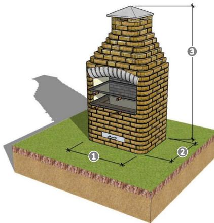
①: A MINIMUM AND MAXIMUM OF THREE (3) FEET IN LENGTH; ②: A MINIMUM OF THREE (3) FEET AND A MAXIMUM OF EIGHT (8) FEET IN WIDTH; ③: A MAXIMUM OF SIX (6) FEET;
